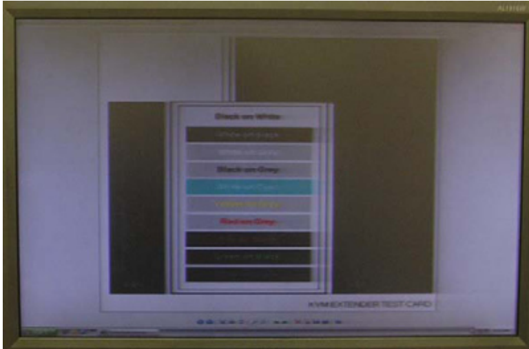
Figure 2. Video image (WXGA @ 60Hz) transmitted over 1000-ft. UTP (CAT5e) cable through Twisted-pair interface.
